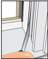
Pry off Monumental Double-Hung jamb liner
